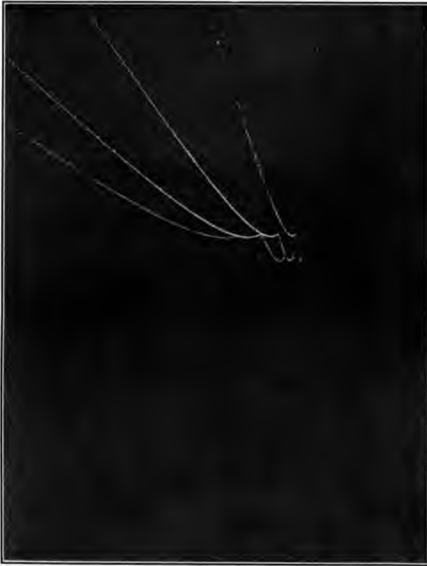
FIG. 165.—Corona at 230 kv. Line A. 3/0 cable. 310 cm. (122 in.) spacing. (Facing page 200.)
